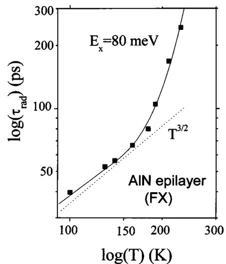
FIG. 5. Temperature dependence of the radiative decay lifetime of free excitons in AlN. The solid line is the fit based on a theory of free exciton dissociation in Ref. 15.
