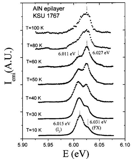
FIG. 2. PL spectra measured at different temperatures for an AlN epilayer. The arrows indicate the PL spectral peak positions of the bound exciton ( $I_2$ ) and free exciton ( $FX$ ) transition lines.
