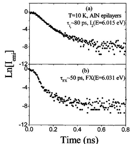
FIG. 3. Temporal responses of PL emissions measured at 10 K at the bound exciton and free exciton spectral peak positions in an AlN epilayer.
